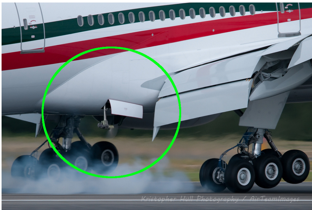
Figure 4: Ram Air Turbine (RAT) and its hatch have been deployed
