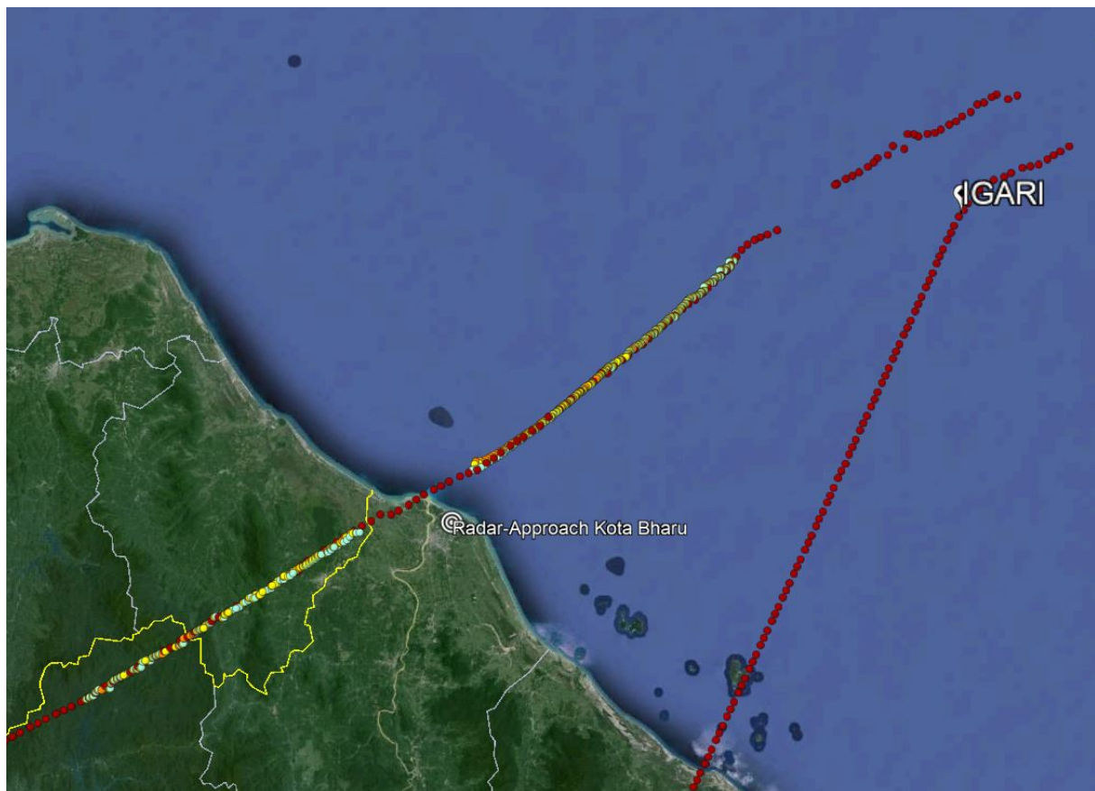
Figure 93: Geoscience data (red) and Kota Bharu PSR data (FL0 white, FL250 Orange, FL300 yellow and FL380 blue)
