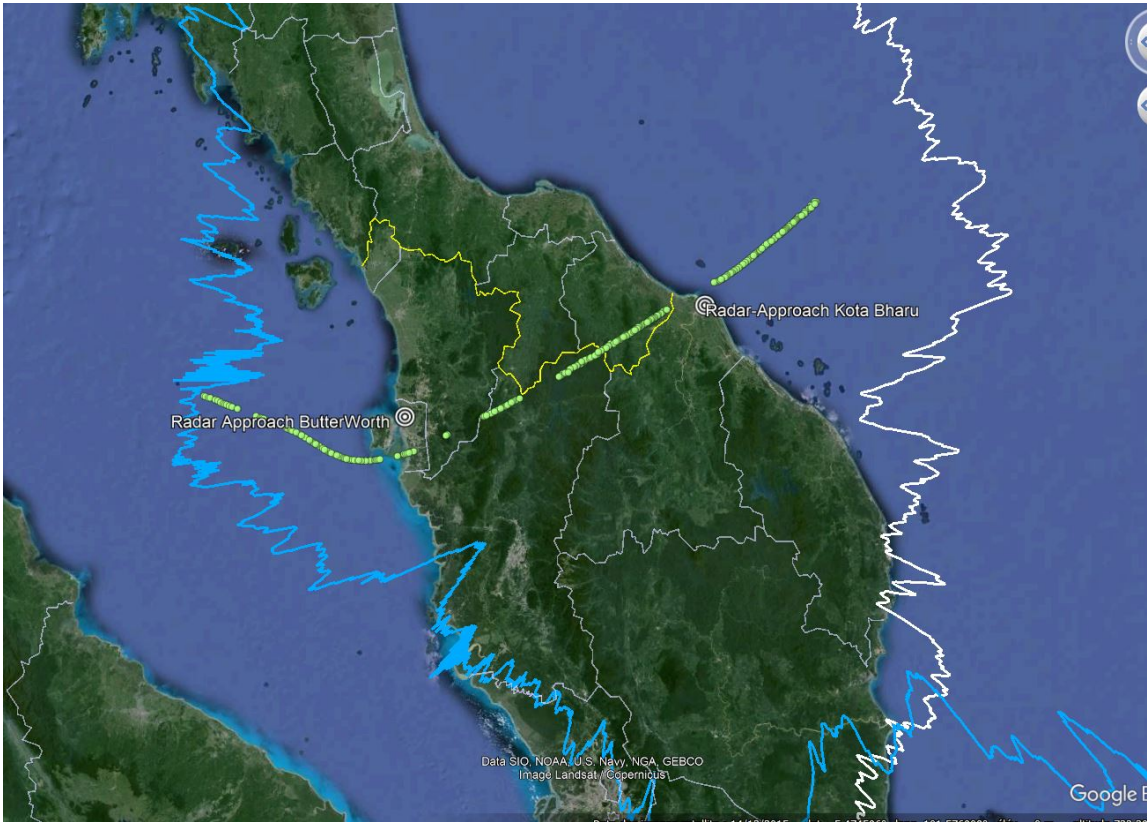
Figure 47: Civilian Approach radar echoes (light green dots) received at Kota Bharu and Butterworth stations
