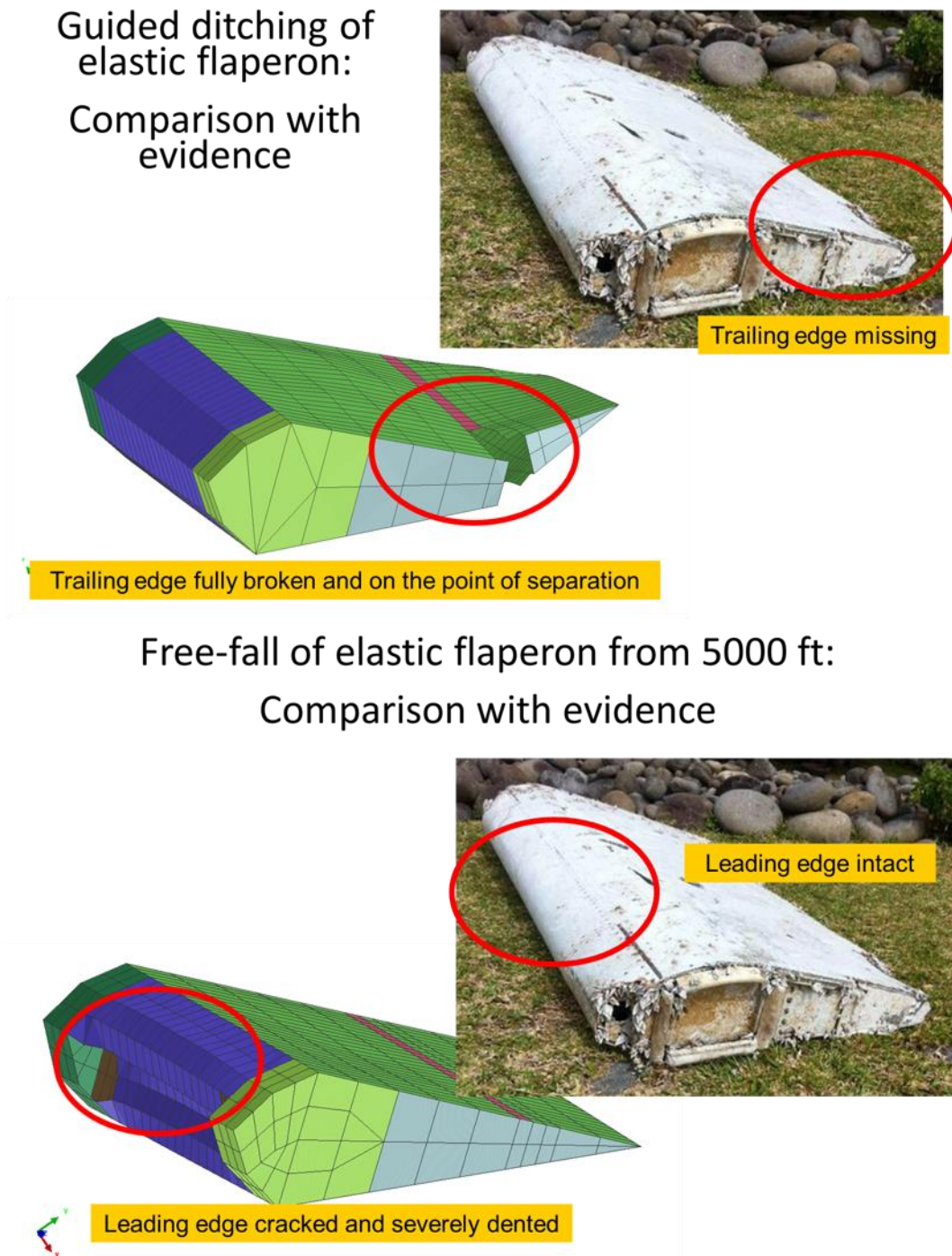
Figure 14: Comparison of consequences on an elastic flaperon between the ditching and free fall impact scenarios upon the sea
